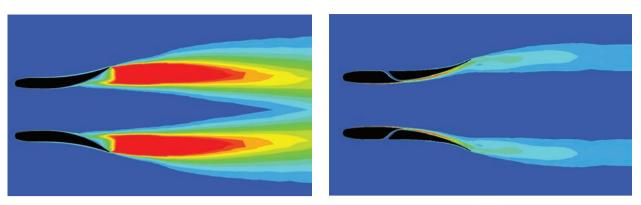
Turbulent kinetic energy plotted over this shroud design shows that flow separates from the diffusor. Inefficient power generation (left) and efficient power generation (right).
