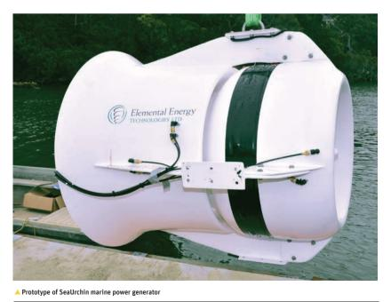
was contracted to evaluate the concept, accelerate design assessment and optimize the design. Engineers employed ANSYS computational fluid dynamics (CFD) simulation, which made it possible to considerably improve the output and significantly reduce development time over standard build-and-test methods.
