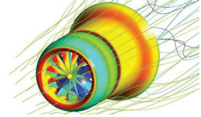
CFD results show pressure plotted on the surface of the power generator with velocity streamlines.
